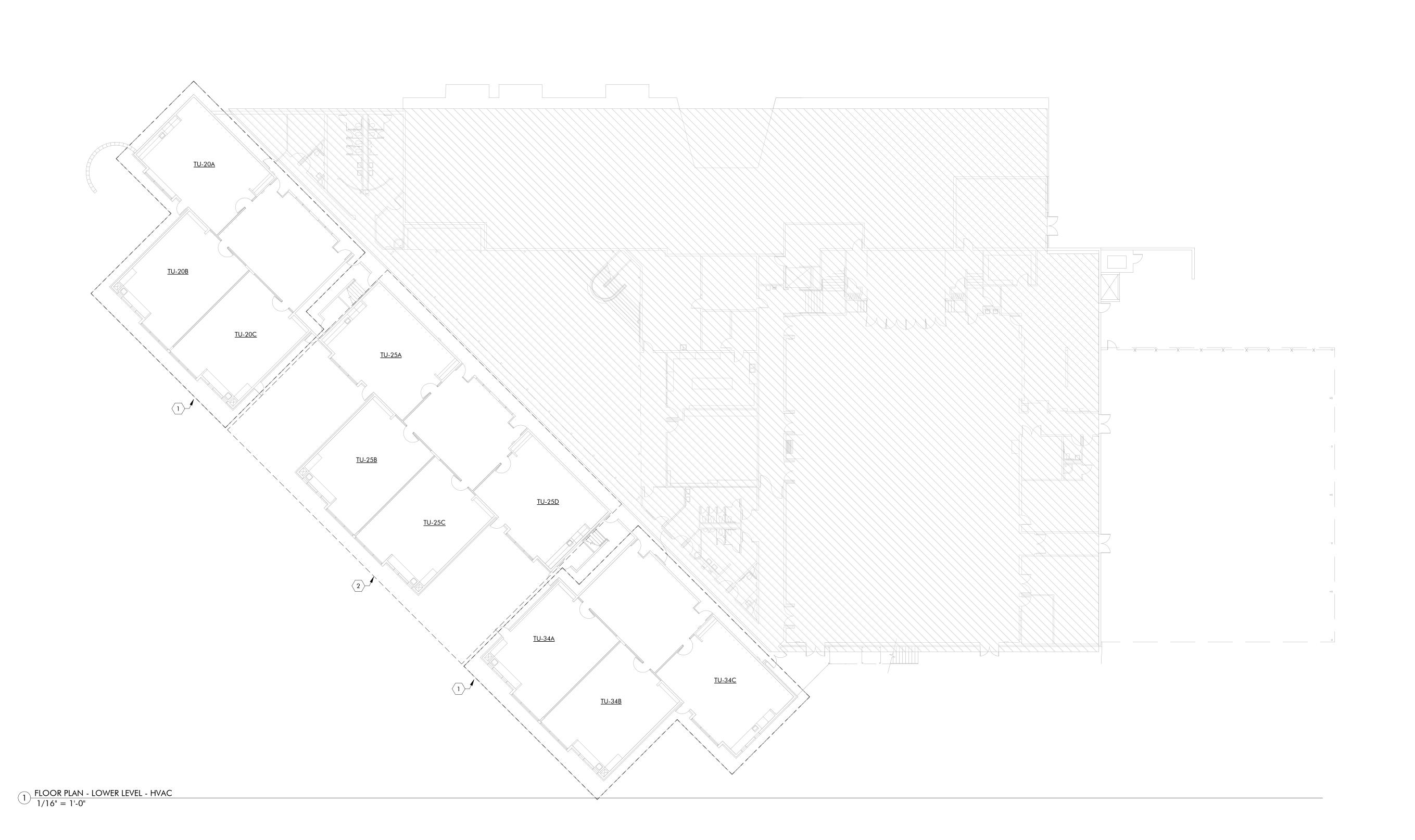
FOR THIS CLASSROOM BLOCK, EXISTING TERMINAL UNIT SERVING (3) CLASSROOMS TO BE REPLACED WITH (3) INDIVIDUAL TERMINAL UNITS AS SCHEDULED ON SHEET M001. SEE SHEET M123 FOR TYPICAL EXAMPLE OF WORK.
