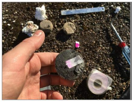
Figure D.38 Moist asphalt-impregnated vapor barrier.
