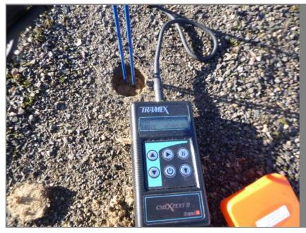
Figure D.62 MC of 9.2% recorded at wood.
