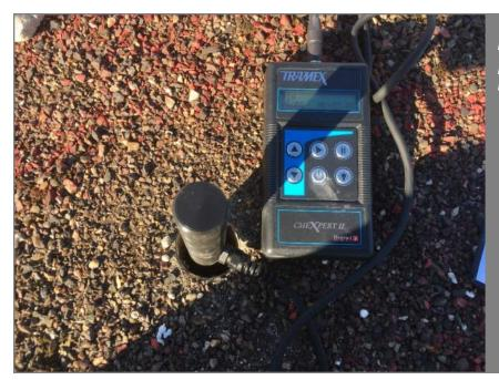
Figure D.35 MC of 33.8% recorded. Plywood soft and deteriorated.
