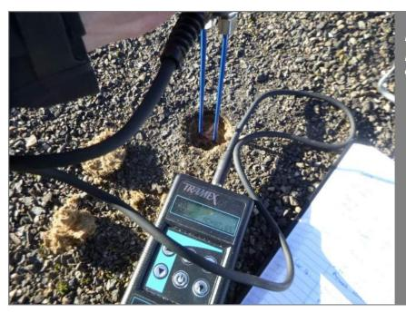
Figure D.59 MC of 7.6% recorded at wood deck.
