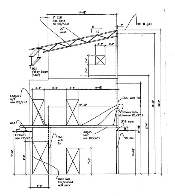
Masonry Wall Coordination Drawing (example only)l
