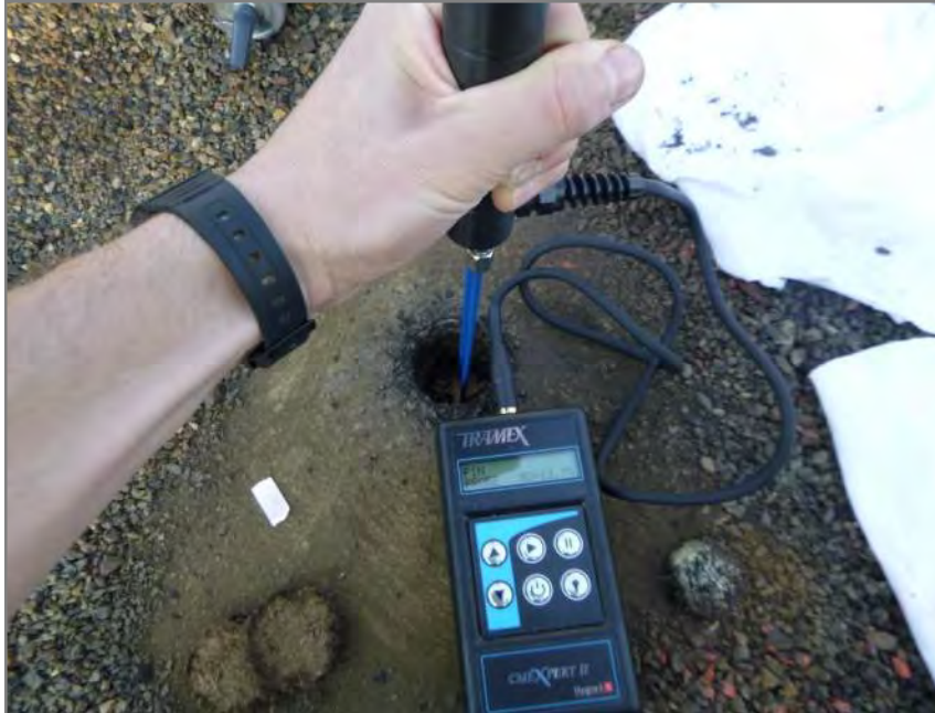
Figure D.19 MC of 12.7% recorded at plywood deck.
