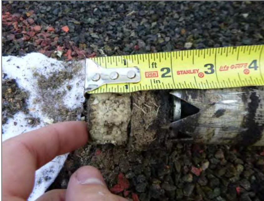
Figure D.7 Typical roof assembly. ½" BUR membrane ½" fiberboard 1" paper-faced Polyiso Asphalt impregnated felt vapor retarder Plywood deck
