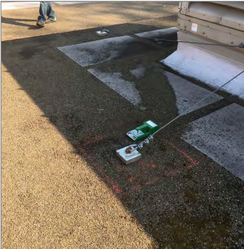
Figure C.6 Core #2 within moisture location #1. Electric impedance reading indicates moisture beneath the surface.
