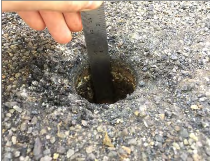
Figure C.15 1/2" BUR 1/2" fiberboard 2-1/2" polyiso insulation Plywood deck
