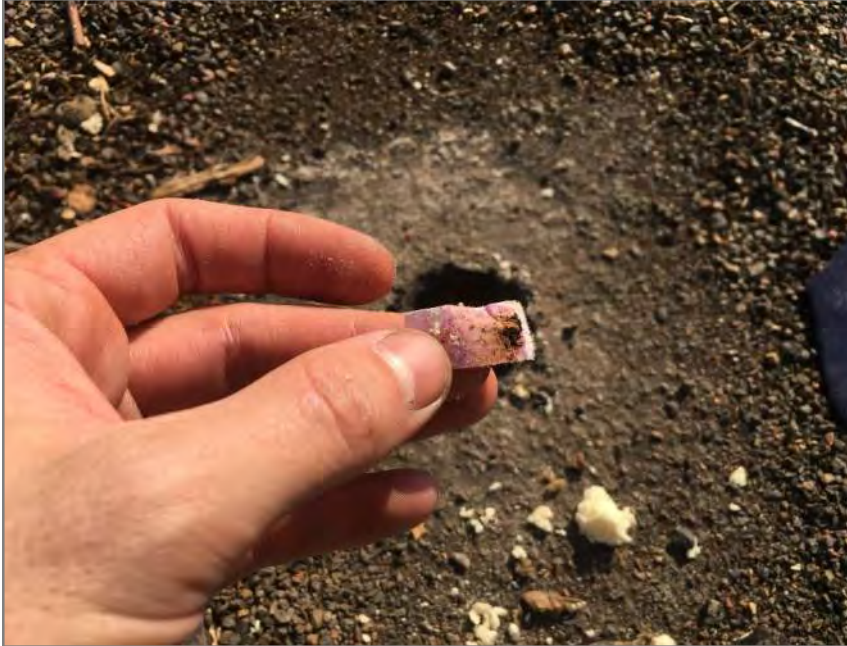
Figure C.5 Moisture identified in insulation by using water reactive paper tape.
