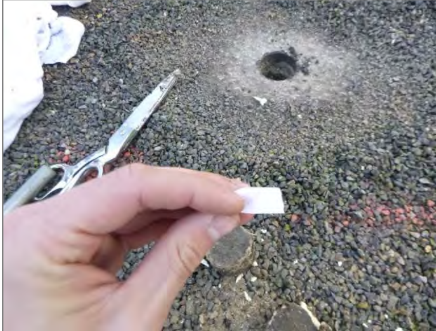
Figure D.13 Moisture present within fiberboard.
