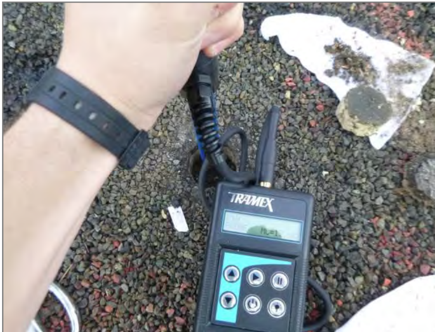
Figure D.10 MC of 12.4% recorded at the plywood deck. Plywood deck is in good condition.
