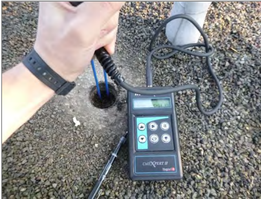
Figure D.14 MC of 14.4% recorded at plywood deck.
