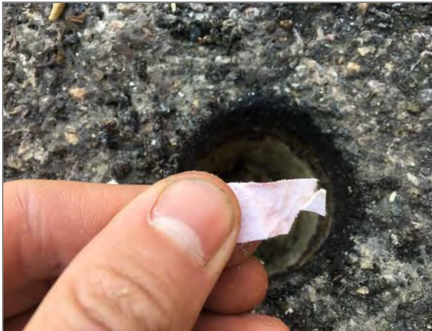
Figure C.8 Moisture identified between insulation and concrete decking.
