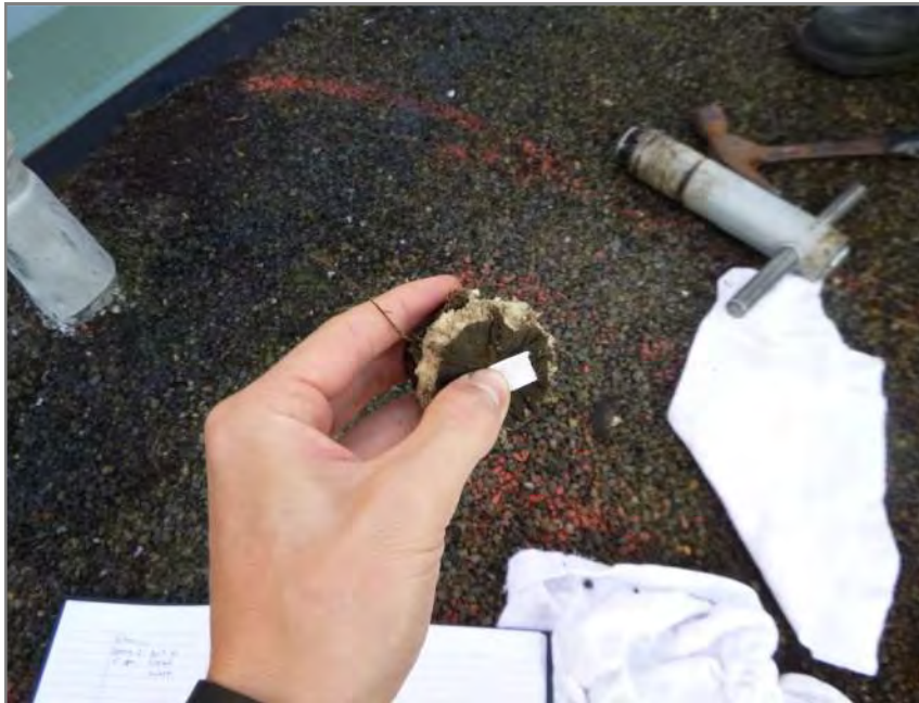
Figure D.2 Moisture present within polyiso insulation.
