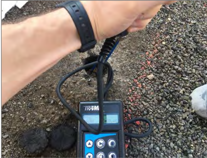
Figure D.23 MC of 25.4% recorded at plywood deck.
