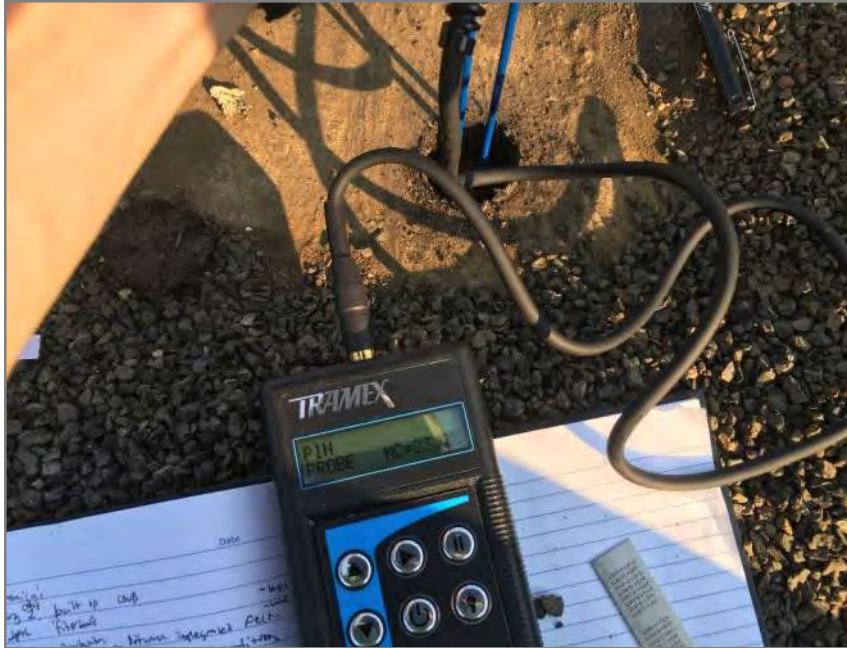
Figure D.33 MC of 23.2% recorded at plywood deck.
