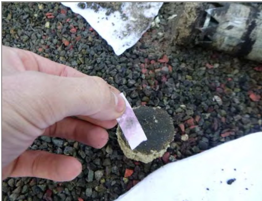
Figure D.8 Moisture present within polyiso insulation.
