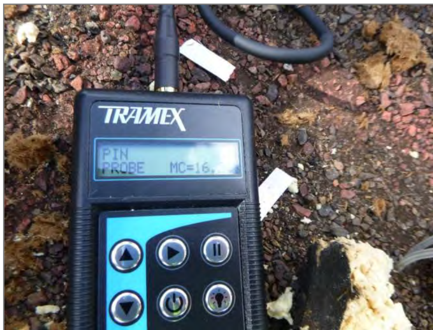
Figure D.17 MC of 16.2% recorded at plywood deck.
