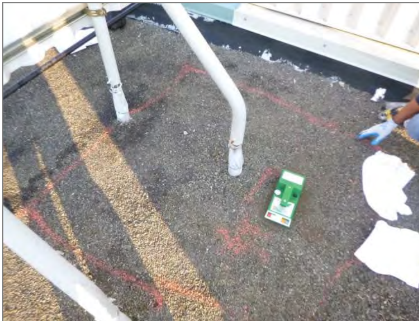
Figure D.20 Electric impedance reading indicates high moisture content within roof assembly at location of core #5 within moisture location #7.
