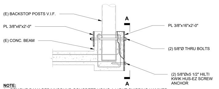
REMOVE DAMAGED/UNSOUND CONCRETE USING A LIGHT CHIPPING HAMMER. PATCH OR FORM AND RE-POUR USING HIGH-STRENGTH NON-SHRINK GROUT.
