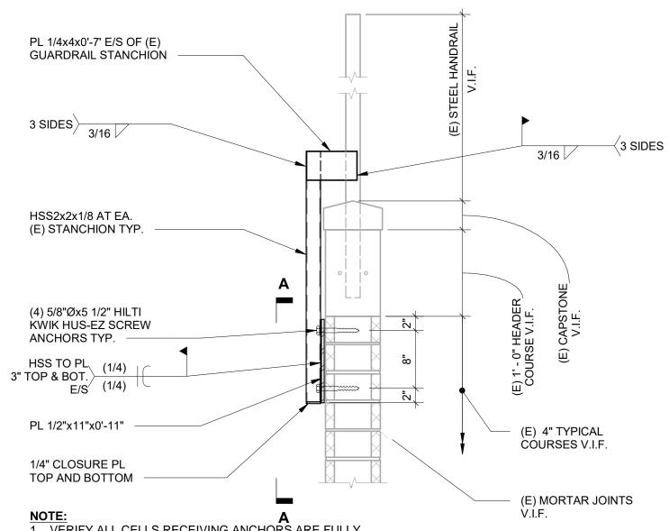
1. VERIFY ALL CELLS RECEIVING ANCHORS ARE FULLY GROUTED. REPAIR AND REPLACE DAMAGED OR MISSING GROUT.
