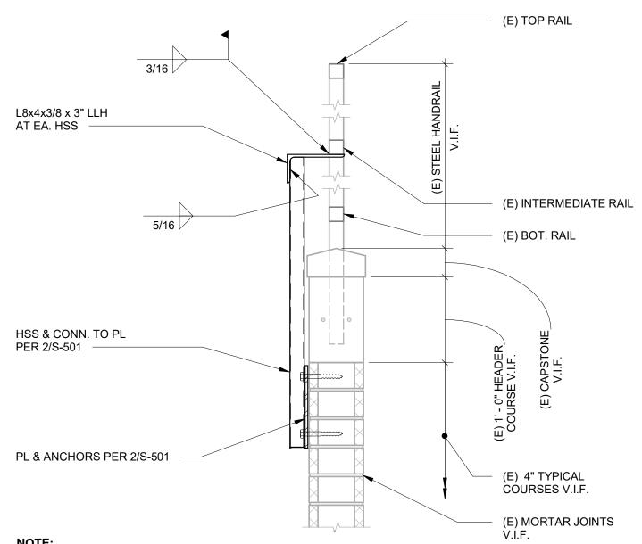
1. VERIFY ALL CELLS RECEIVING ANCHORS ARE FULLY GROUTED. REPAIR AND REPLACE DAMAGED OR MISSING GROUT.
